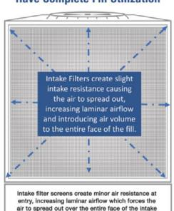
opening — resulting in increased fill utilization and lower water temperature at the basin.
