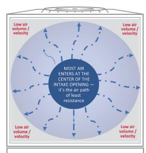
The further away you get from the center of the tower, the lower the air volume and velocity entering the cooling tower fill; upper and lower corners have the lowest air volume and velocity entering the fill.
