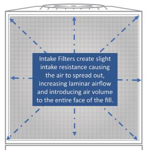
Intake filter screens create minor air resistance at entry, increasing laminar airflow which forces the air to spread out over the entire face of the intake opening — resulting in increased fill utilization and lower water temperature at the basin.
