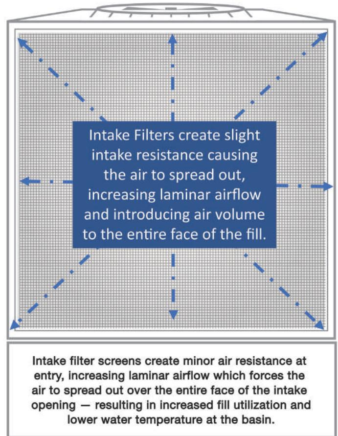
In addition to stopping airborne debris at its point of entry, Cottonwood Filter Screens by design, slightly increases airflow resistance causing the air to spread out over the entire intake opening resulting in an increase in “Laminar Airflow.” In other words, it creates a ‘wall of air’ that fully covers the intake opening thus exposing the entire fill pack to more air volume and velocity versus not using screens and having lower Fill Pack utilization.
